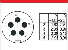
Contact arrangement (Plug-in side)
